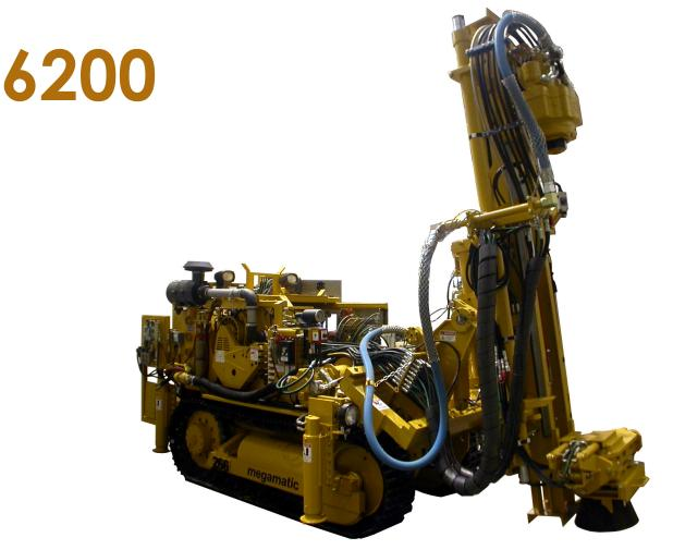
**Description:** The 6200 is a track mounted In-The-Hole drill designed to drill with ITH hammers powered by high air pressure. High pressures are obtained with an optional towable booster.
